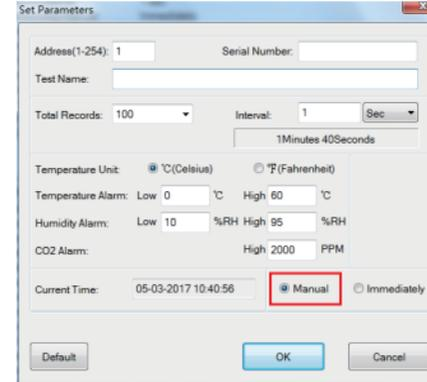
The parameter setting is the same as mentioned above. The difference is that we will select manual measurement. After completion of the setting, exit and plug off the data line and take the instrument to the destination. Press “REC” key on the instrument to begin recording the data. After we bring the instrument back and connect it with a computer, click “ Data Download”. The data we received is the data we measured and record outdoors.
