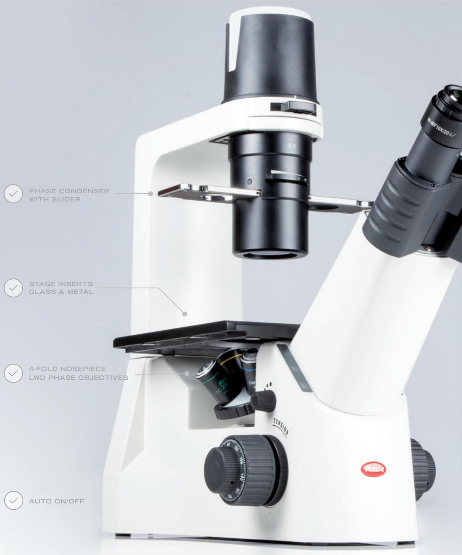
optional 4X Phase objective is dedicated to fast screening. A 40X Phase objective is available too. The AE2000 stand carries a quadruple nosepiece with a precise click stop. Rich illumination power is given by the 30W Halogen light source in a Fixed-Koehler setup, simply interchangeable with 3W LED modules of different color temperatures. The Auto ON/OFF function is a contribution to workplace safety.
