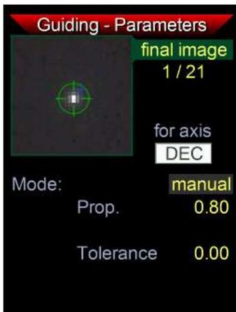
On the DEC page the standard mode is currently **manual** only. The DEC shows neither periodic error nor overtones, but static drifts or erratic movements. So an integral term does not make much sense. Instead, a value of 0.8 for proportional will suit most situations. In the case of overreaction you may lower this value to avoid oscillation of the mount. The tolerance can be left at 0.00, or increased if corrections in the DEC axis need to be dampened. For advanced users only!
