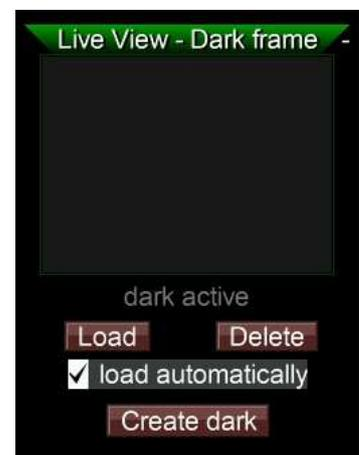
The corrections are applied, **dark active** is displayed and the file is saved onto the SD card. If there is no SD card in the slot, there is a warning, but the corrections remain active until shutdown.
