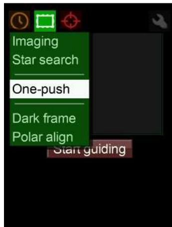
Here you can shift the cursor by pressing the directional buttons **UP ▲** and **DOWN ▼**. By **LEFT ◀** and **RIGHT ▶** you can change to other main menus.
