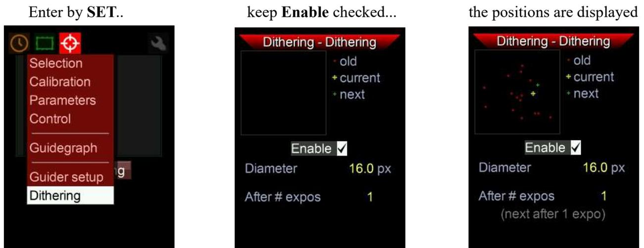
If enabled, the MGEN-3 will shift the guide star automatically a little bit after the specified number of exposures. You can observe the shifting on the active LEDs of the directional buttons when the ST4 output is activated immediately after the DSLR exposure has ended.
