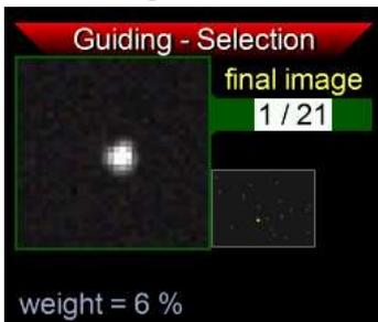
If the cursor is set to the star number and **SET** is pressed, the image of the respective star is displayed (here star 1 from 21), and the weight for its contribution to the multistar. The smaller window shows its position on the sensor.
