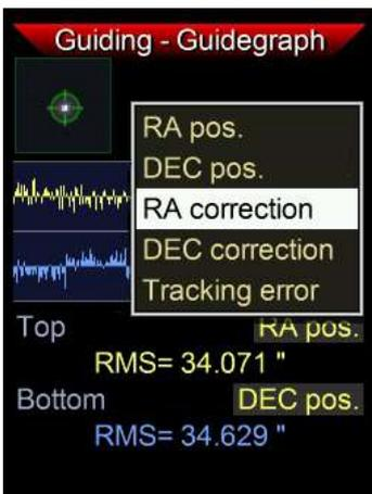
If the cursor is on **RA pos.**, you may press **SET** and a box pops up. Here you can choose what kind of graph should be displayed – correction means the length of the respective AG signals, and tracking error are the summarized corrections.
