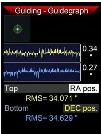
By default you see the positions of the multistar displayed, showing the deviations from the zero line. RA is the upper, DEC the lower graph. The graph is updated every guide cycle and shows about the last 220 positions.
