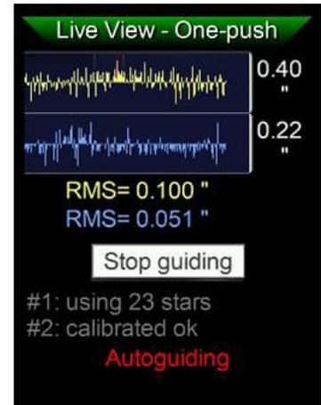
The live image is replaced by the guide graph, showing the progress of the autoguiding and displaying the rms deviations. You may also stop and resume guiding from here. If a new starfield is detected, a new star search and calibration takes place automatically. If detection fails, you may go to the Star search page and start the Star search there manually. Normally, the whole one-push sequence from start to autoguiding takes only about 30 seconds, no more.
