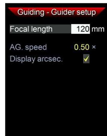
Check if the default values fit or need to be corrected for your setup. A 50mm finder usually has a focal length of 180mm, and a 30mm finder is usually 120mm. A Synta 50mm ED finder has 240mm.
