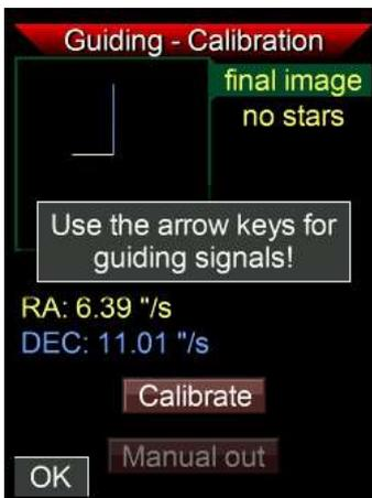
At the bottom of the page there is the **Manual out** button. This is an important tool to check the connection to the mount. Set the cursor and press SET, a box appears telling you to now transmit the ST4 signals by pressing the directional buttons. Check if the multistar moves when you output the signals manually. Exit this mode by pressing **ESC (OK)**.
