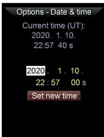
The MGEN-3 has a real-time clock built in, that is powered by an internal battery and continues even after shutting down. Format is YYYY MM DD
