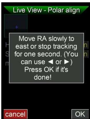
A box pops up. Simply follow the instructions. Your mounts RA axis needs to be slowly moved a little eastwards. You may use the **RIGHT** (or **LEFT**) button on the MGEN-3 to manually send the respective ST4 signal, or you can stop tracking for a few seconds, and then press OK. A little line appears, stretching from the multistar pointing to the pole.
