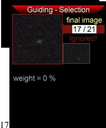
Using the buttons **LEFT** and **RIGHT** the stars can be called up one by one, and deactivated or reactivated by pressing **SET**. A deactivated star is shown against red and is ignored, and its weight is set to 0%.
