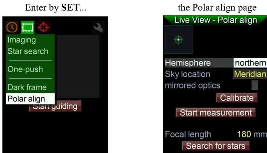
Polar aligning a mount usually is done before autoguiding, so after startup you can switch directly to this page. Set the focal length of your guidescope, if not already done. We recommend to start with a star near the meridian. That helps later on to eliminate the height error as the azimuth is already fine tuned).
