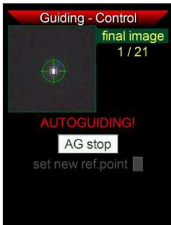
When autoguiding is started, **AUTOGUIDING!** appears and blinks, and a red cross marks the set point where the star should be kept.
