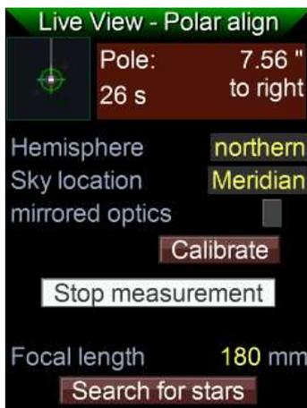
After a few seconds, results appear that are continuously updated as time goes on. The deviation is displayed in size and direction. Wait for about 30 seconds until the number gains stability, stop the measurement and correct the azimuth of your mount. If the pole is to the right, your pole block must also be turned to the right, (clockwise, as seen from above).
