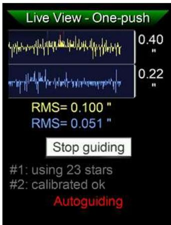
The live picture is then replaced by the guide graph, and at the bottom, Autoguiding is displayed in red blinking letters. You may now start the exposure sequence with your camera.
