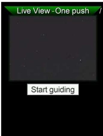
To set the cursor on **Start guiding**, push the **DOWN ▼** directional button, and then press **SET** (from firmware 1.01 the cursor will be on **Start guiding** by default).
