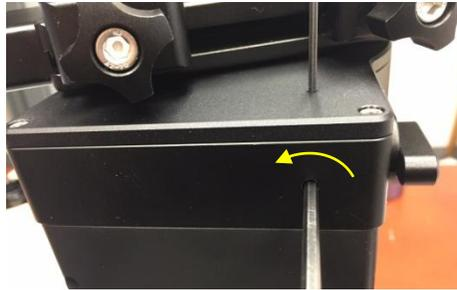
If the motor stalls or the mount does not tracking smoothly, most likely the meshing is too tight. You may loosen it by about 1/8 turn (or less for tracking). **Tighten the set screw in the small hole to LOCK the gear screw (important) before test the mount.** Adjust again if needed, but no more than 1/4 turn in total.
