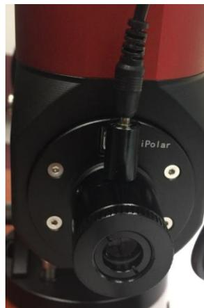
Figure 24. Connect polar scope LED
