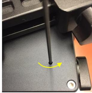
Adjust the **gear adjustment screw** on the side inside the large hole by using the 3mm hex key. Turn counterclockwise to loosen the meshing or turn clockwise to tighten the meshing.
