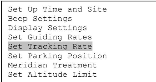
Then the user can select “**Sidereal Rate**”, “**Lunar Rate**”, “**Solar Rate**”, “**King Rate**”, and “**Custom Rate**”. The “**Custom Rate**” can be adjusted from 0.9900X to 1.0100X of sidereal.
