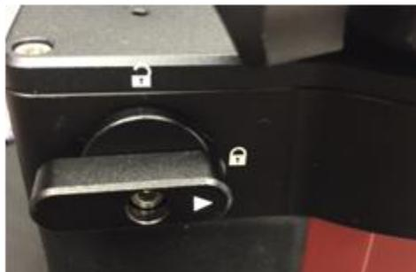
Insert the 2mm hex key into the small hole on the top. Gently turn the hex key until you feel it is engaged to the set screw inside. You may turn the gear switch further in the lock position if the wrench can't engage the set screw. Turn the **set screw** half a turn counterclockwise to release it.
