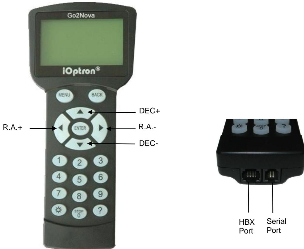
Figure 7. Go2Nova<sup>®</sup> 8407+ hand controller
