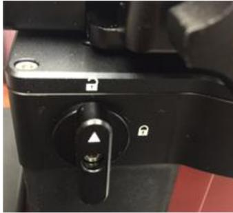
Rotate DEC saddle to exposure the small hole (3mm in diameter) that is blocked by the dovetail saddle. Another larger hole (5mm) is located on the side of the DEC gear housing. There is a **set screw** inside the 3mm hole which locks the **gear meshing adjustment screw**, which is inside the larger hole.
