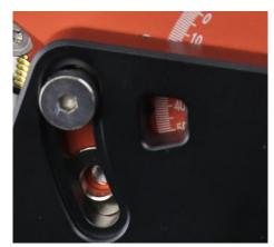
Unthread and remove the Position Bolt to its new location. Adjust the Latitude Adjustment Knob while holding the brass eyebolt until it lines up with the Position Bolt. Secure the Latitude Position Bolt.
