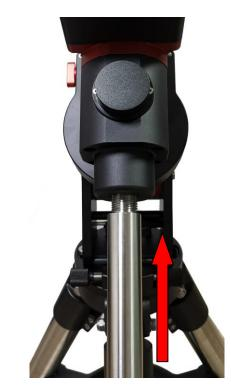
5. Install Counterweight(s): Before putting on CW, make sure the mount is at its zero position, i.e., CW shaft points to the ground. Disengage the R.A. Gear Switch to set the R.A. axis free before loading the CW. Remove the CW Safety Cap at the end of CW Shaft. Glide the CW over the shaft. Tighten the CW Locking Screw to hold the CW in place. Place the Safety Cap back onto the shaft. Move the CW to the bottom of the shaft and tighten the CW locking Screw.
