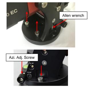
Level the mount by adjusting the tripod legs. Use the build-in bubble Level Indicator or an external leveler for this purpose.
