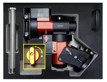
2. Set up Tripod: The tripod top is 120 mm in diameter with 2x M6 holes 103 mm apart for mounting. Two additional M6 holes are for the Alignment Peg (the one right next to one of the legs is for uses at high latitudes; the other one is for uses at low latitudes). Thread the Alignment Peg into the correct M6 hole. Insert the Accessory Tray through the center rod and secure the setup by tightening Locking Knob from underneath.
