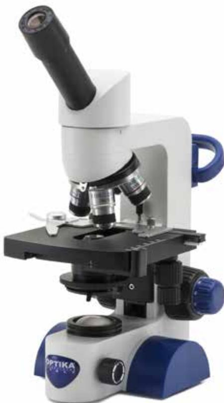
Cordless, modern monocular microscope ideal for students and mainly primary schools with achromatic lenses (1000x), FN 18, finite optical system, coaxial focusing, StagErase™ erasable mechanical stage and 1 W LED illumination with rechargeable batteries. Slim and easy to carry, it is equipped with arm /wrist rest support to reduce the fatigue during use and long lasting LED illumination to provide over 20 years of use.
