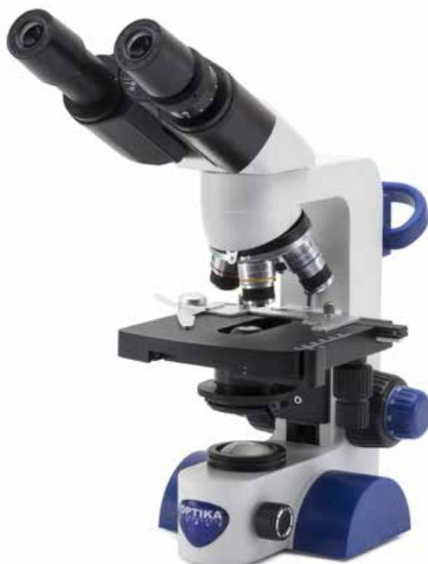
Cordless, modern binocular microscope ideal for students and mainly primary schools with achromatic lenses (600x), FN 18, finite optical system, coaxial focusing, StagErase™ erasable mechanical stage and 1 W LED illumination with rechargeable batteries. Slim and easy to carry, it is equipped with arm /wrist rest support to reduce the fatigue during use and long lasting LED illumination to provide over 20 years of use.
