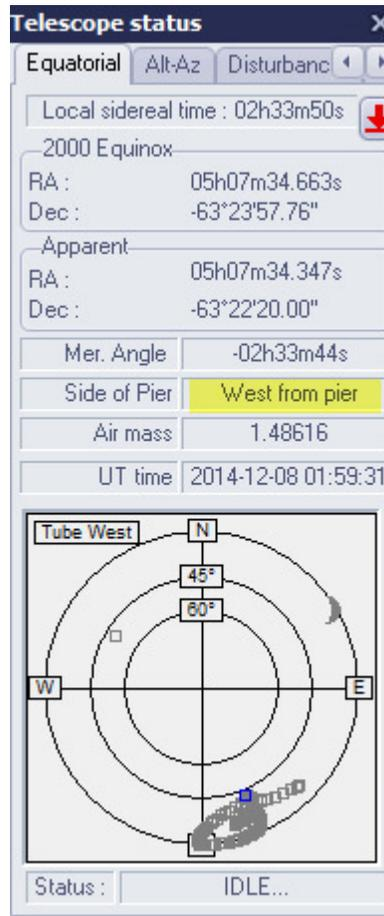
The idea is to have the telescope to scan this area with many fields, perform plate solving and create a list that contains the actual telescope position and theoretical (or expected) position. To obtain a good pointing model, this scan must have regularly sampled fields across the sky, and at least 20 fields (40 is better).
