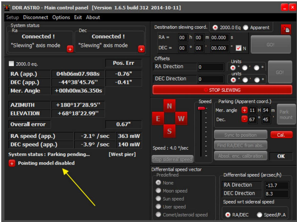
Go to **“Setup”** then **“System setup”**, press **“German mount setup”** and change as follows the allowable mount clearance.
