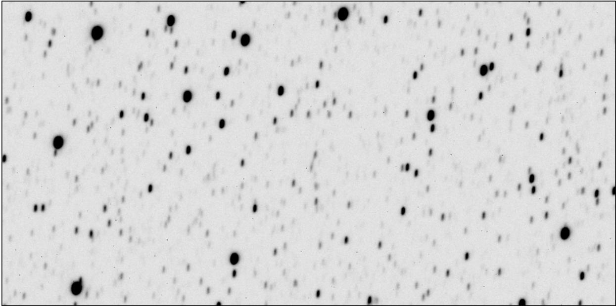
The image quality is weak and shows a vertical trailing in DEC direction. This is quite normal with badly polar aligned mounts.
