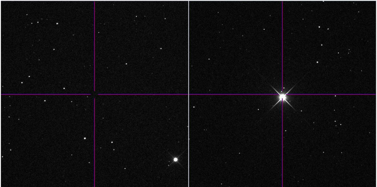
Working without a pointing model can allow dramatic errors with a German mount. Meridian flip and optical axis non perpendicularity error with the DEC axis can lead to pointing errors more than  $\frac{1}{2}$  of a degree! This causes most of the time, the target to be outside the field of view of the camera. A Pointing model can overcome this easily, allowing better use of your telescope, and not wasting time acquiring your target.
