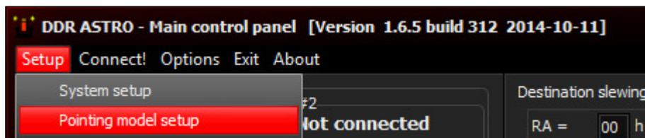
Enable pointing model and select the **TubeWestPier-10-10-14.cor** and **TubeEastPier-10-10-14.cor** accordingly. So having named the files this way is a good trick to avoid mixing up these files.
