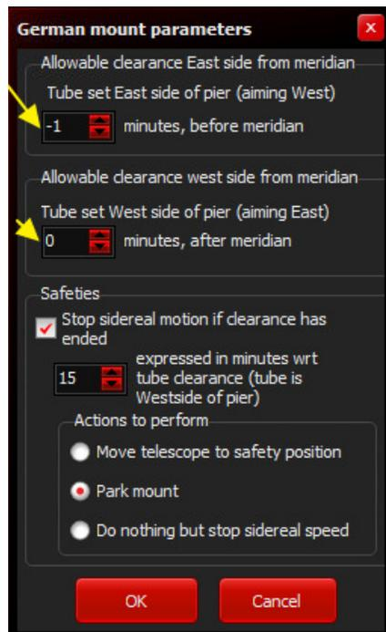
This step is achieved to avoid unwanted meridian flip, because two pointing models are required for German mounts, **one for the tube located at the east side of pier, and another for the west side of pier.** Since pointing models are created by slewing to areas only in one side of the pier, these settings forbids the mount from meridian flipping when located close to the meridian.
