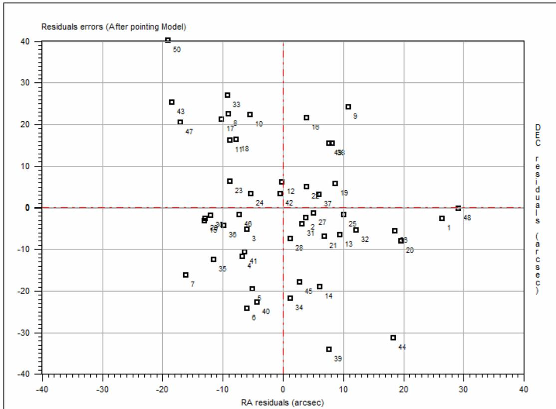
Even more impressive is the “**Projection errors**” tab showing errors before and after pointing model
