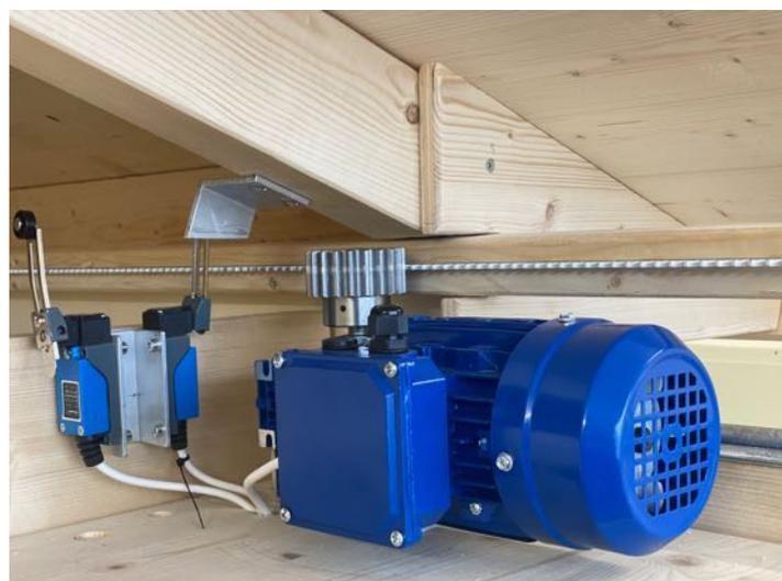
The roof drive is installed on the left-hand side of these **GreenLine RollOff observatories**.
