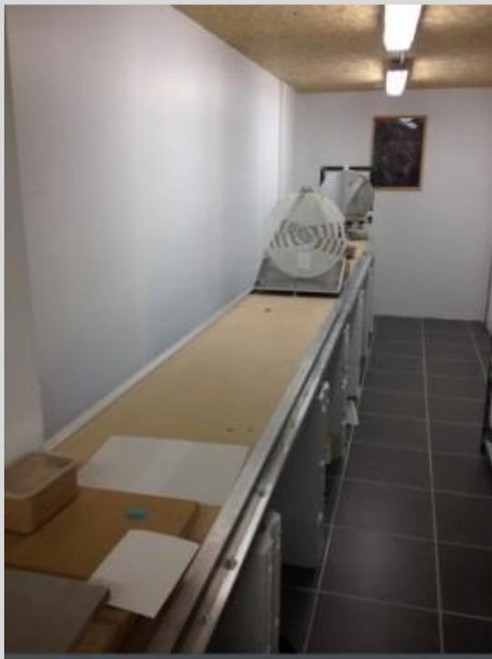
*Our workshop is equipped with a test bench of 6 meters long mounted on anti-vibration isolators.*
