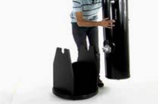
1. Remove the telescope tube from the base and set it aside for the moment. You will be working with the base.
