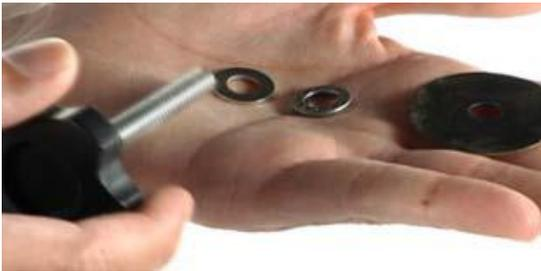
a. Unscrew the center Adjustment Bolt and remove it, including all washers and bearings. Set aside, they won't be needed.
