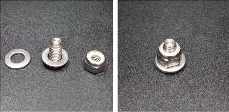
13. Put the 5/16 SAE Stainless Washer (d) on top of the Flanged Sleeve Bearing and secure with the 5/16-18 Nylon Insert Lock Nut (c).
