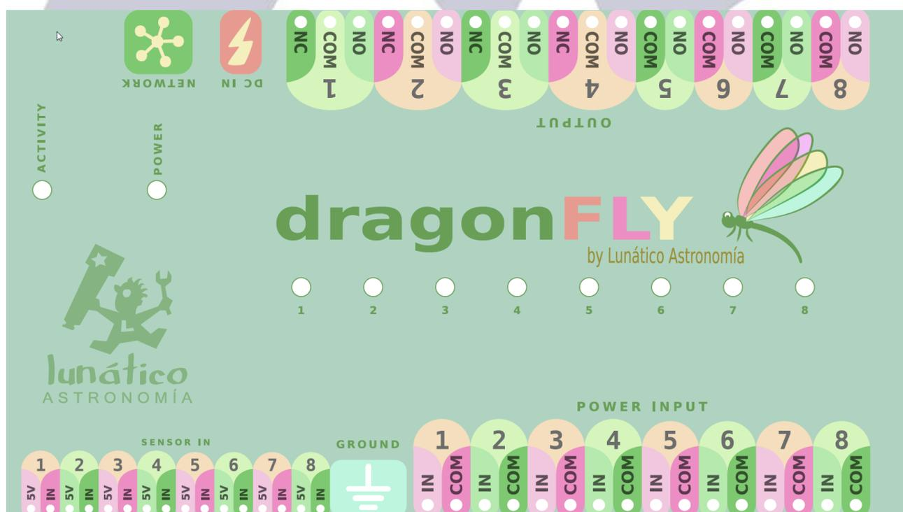
... you'll note we've used this naming convention for labeling the input and output connectors.
