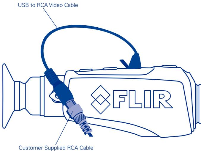
When using the USB/Analog Video Adapter cable to record video or supply video to a remote monitor, it may be useful to turn off the Auto Power Off feature of the monocular.
