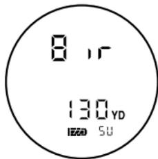
last saved distance, until 200 yards (185 meters) has been reached. Once 200 yards (185 meters) has been reached, it will reset to 60 yards (55 meters), and start over again. When the appropriate distance is displayed, press MODE.
