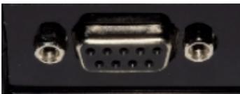
The controller is fitted with a D Sub 9 Pin Female Connector.
