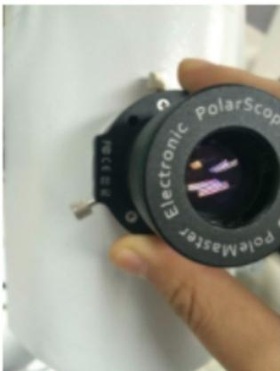
When not in use, you can either leave the camera on the mount attached; alternatively, you can remove the camera (with its camera base disc) from the mount ring by loosening the thumbscrew. Always protect the camera lens using the screw-on lens cap when not in use. If you choose to remove the camera, you may also want to prevent ingress of dust, dirt, bugs, etc into the mount through the mount ring by covering the mount ring opening with the adaptor cap provided.
