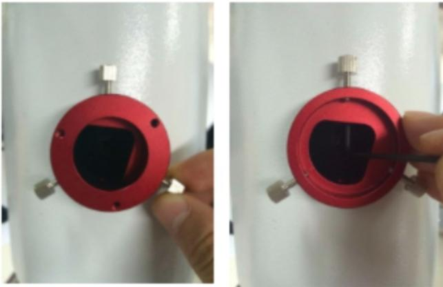
Attach the camera disc to the back of the camera body using the bolts provided. You only need to perform this step on your first use.
