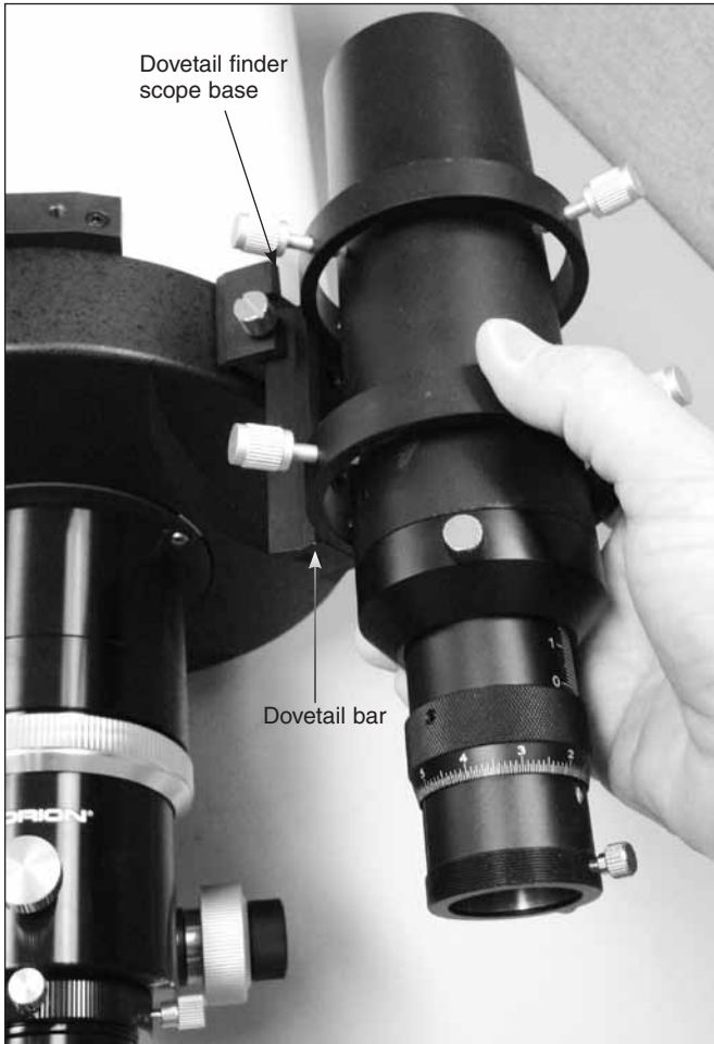
Figure 2. The guide scope bracket's dovetail fits Orion dovetail finder scope bases as well as those of some other manufacturers.
