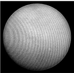
Another effect present in CCD imaging of monochrome light of Hydrogen Alpha or Calcium H is the interference pattern - or Newton's Rings.
