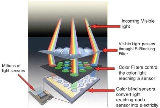
The imager should also appreciate that even after considering IR blocking filters, that the COLOR CCD chip is constructed in a way that only 1 in 4 pixels detect red light. The other 3 sensors only detect blue and green because the pixels are actually permanently covered with a colored dye for each corresponding color. So a color CCD chip (in a DSLR or a CCD camera) will only offer 1/4 the sensitivity and 1/2 the resolution of a monochrome chip.
