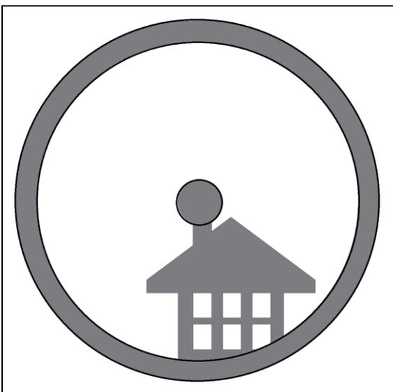
**4.3.** After playing with the two adjusters and some trial and error we get the finderscope reticle close to the center (in this case the chimney). The finderscope is now ready to use!
