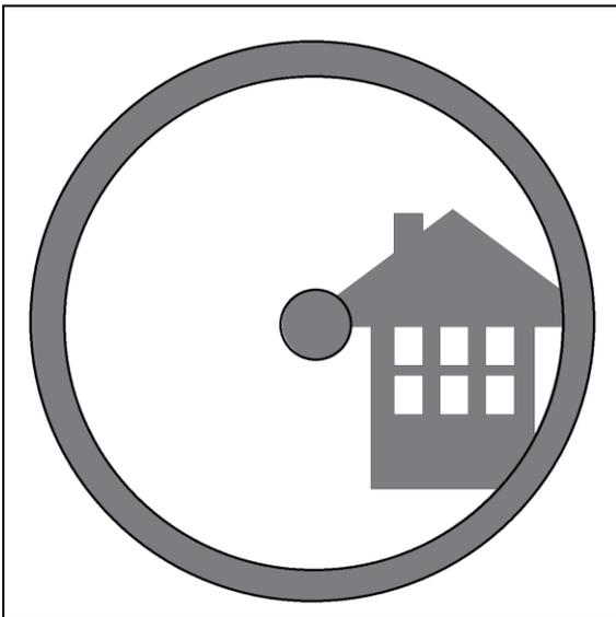
**4.2.** Looking through the finderscope (it should be powered on) we see the same building but in this case the red dot and chimney are not centered. We adjust the finderscope removing the caps from the adjusters so that the finderscope's red point moves slightly until it matches the chimney. This is enough to correct the objects position in the finderscope. Trial and error is required to get a satisfactory result.
