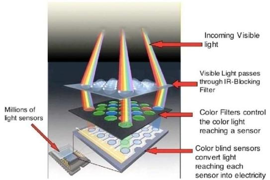
The DSLR imager must be aware that most camera manufacturers (Canon and Nikon) use an IR blocking filter which greatly reduces the transmission of Hydrogen Alpha light. DSLR cameras without this IR blocking filter will have better sensitivity imaging in Hydrogen Alpha.
