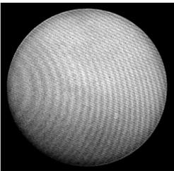
Another effect present in CCD imaging of monochrome light of Hydrogen Alpha is the interference pattern - or Newton's Rings. The effect is similar to interference testing of an optical surface between two flat surfaces. The sensor and cover slip cause a small interferometer inside the camera and cause a Newton's Ring moiré' pattern. The CCD chip must be tilted to a minor degree to prevent this pattern. Recent advances
