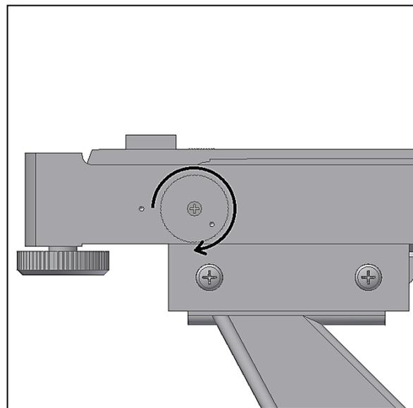
Figure 3. Turn power ON by rotating potentiometer.
