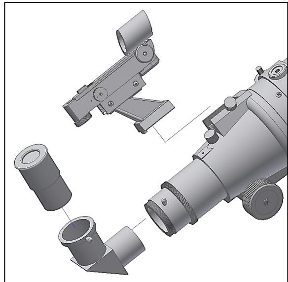
Figure 9. Place finderscope and eyepiece at the telescope.
