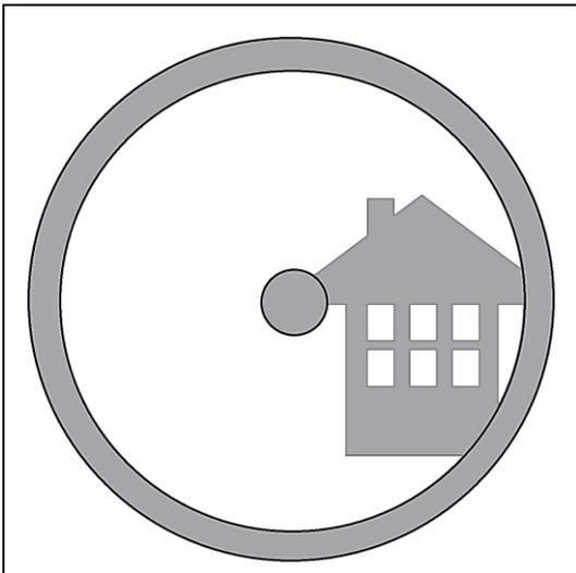
**3.2.** Looking through the finderscope (it should be powered ON) we see the same building, but in this case the red dot and chimney are not centered. We adjust the finderscope using the two altitude and azimuth knobs so that the finderscope red point moves slightly until it matches the chimney. This is enough to correct the objects position in the finderscope. Trial and error is required to get a satisfactory result.
