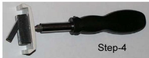
5-6. Teflon pad with block unit to be inserted into the new Lacerta pressure plate
