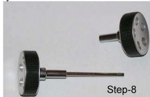
9-10. Insert the original shaft with one knob into the new Lacerta microfocuser unit (do not secure it yet)
