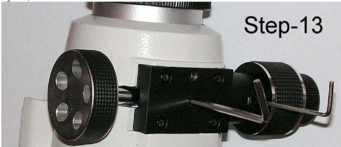
14. Loosen up the gear housing with the right Allen key
