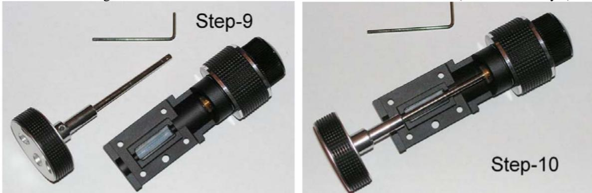
11. Install the new Lacerta microfocuser unit containing the original shaft & knob onto the focuser.
