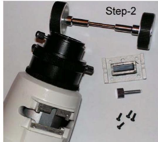
3-5. Remove and keep the Teflon pad together with the block unit
