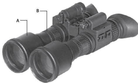
FIGURE 3-7. MOUNTING 3X AFOCAL LENSES TO THE N-15
