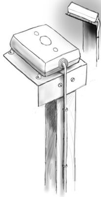
To ease *water evacuation*, the device must be installed slightly tilted (10 to 15° is perfect); it is recommended to make the unit point to the zone from where clouds more usually come, thus allowing for an earlier detection.
