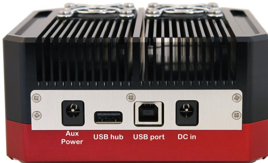
**Aux Power** – 2.1mm center positive socket, for external devices (Max 2A)
