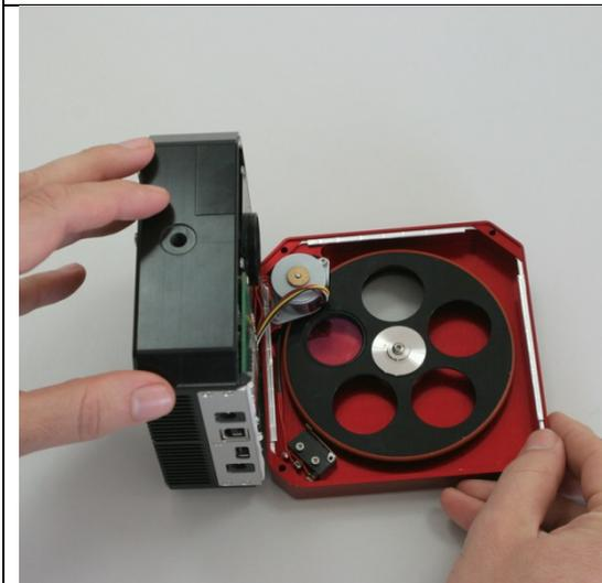
Turn down the wheel module onto the table.
