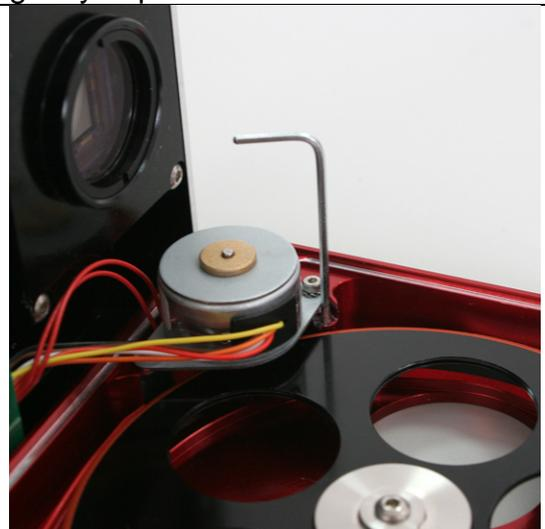
Lock the motor with the supplied 1.5mm Allen key.
