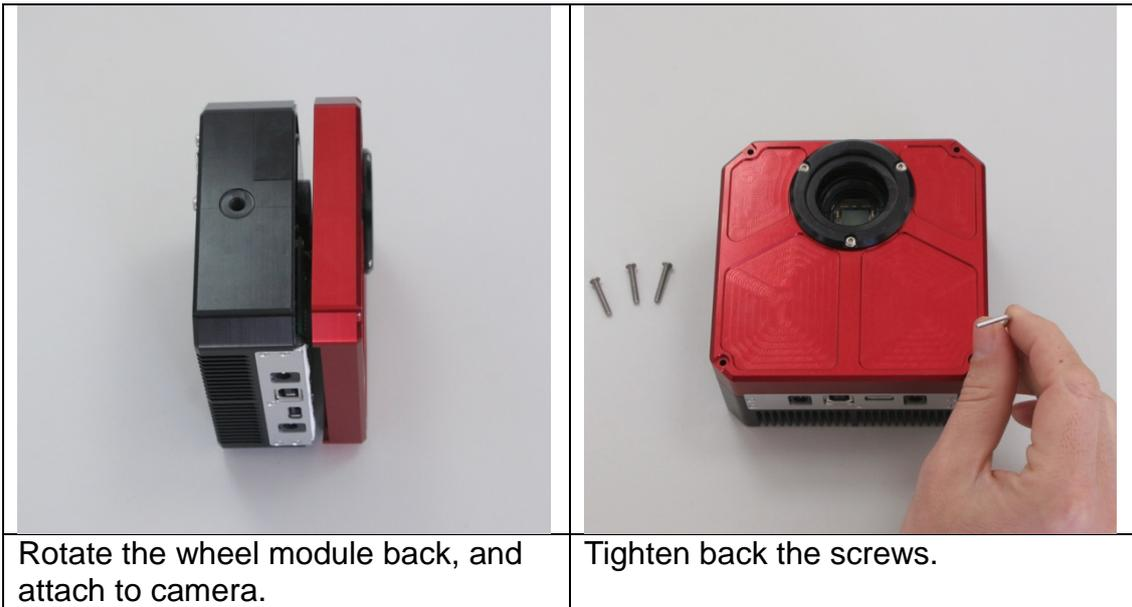
Rotate the wheel module back, and attach to camera.
