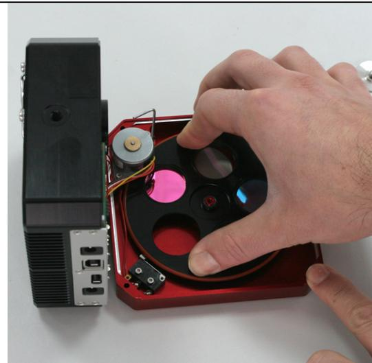
Install disk. Make sure the disk clears the mechanical index on the lower left. If needed, use a pen tip to lower the blade.
