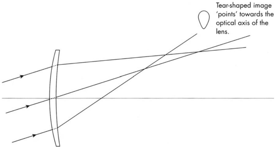
Fig. 2.25 Coma in a converging lens
