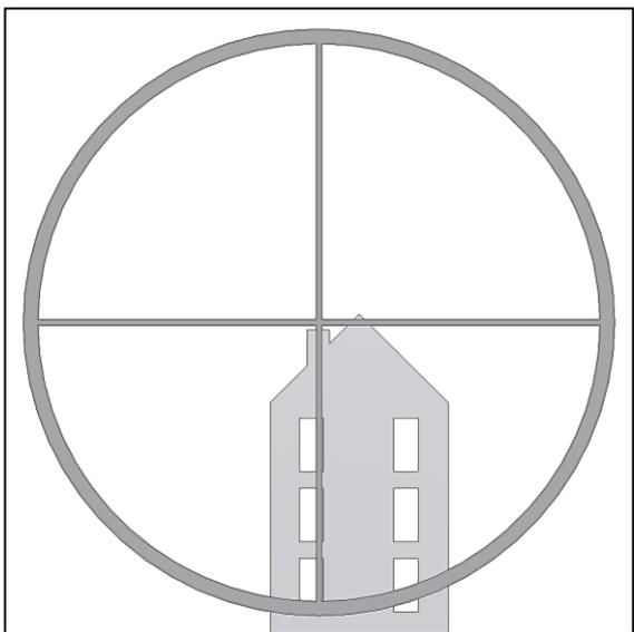
**4.3.** After playing with the three finderscope thumbscrews and some trial and error we get the finderscope's recticle close to the center (in this case the chimney). The finderscope is now ready to use!
