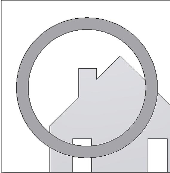
**4.1.** A distant object is centered at the telescope's field of view with an eyepiece. In this example we have a house with a chimney. The chimney is the reference point to place at the center of the field of view. We first look through the telescope with the lowest magnification possible to get the widest field of view.
