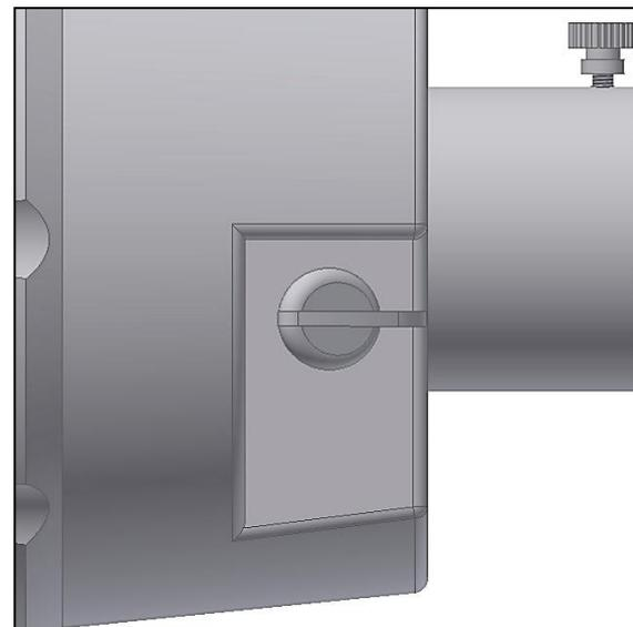
Figure 4. Flip mirror horizontal (light comes through back - #6 suitable for DSLR use).
