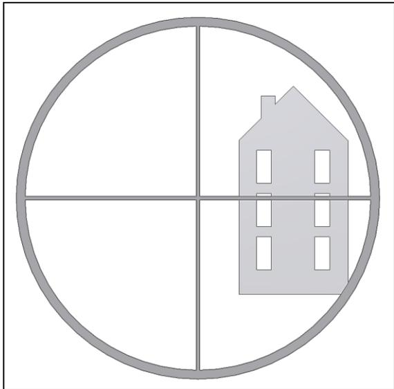
**4.2.** Looking through the finderscope we see the same building, but in this case the chimney is not centered. We adjust the finderscope using the three thumbscrews, so that the finderscope moves slightly. This is enough to correct the objects position in the finderscope. Trial and error is required to get a satisfactory result. Make sure to tighten the 3 screws after finishing, so that the finderscope tube does not move.
