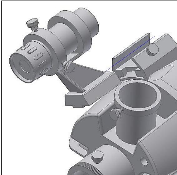
Figure 1. Install the finderscope.
