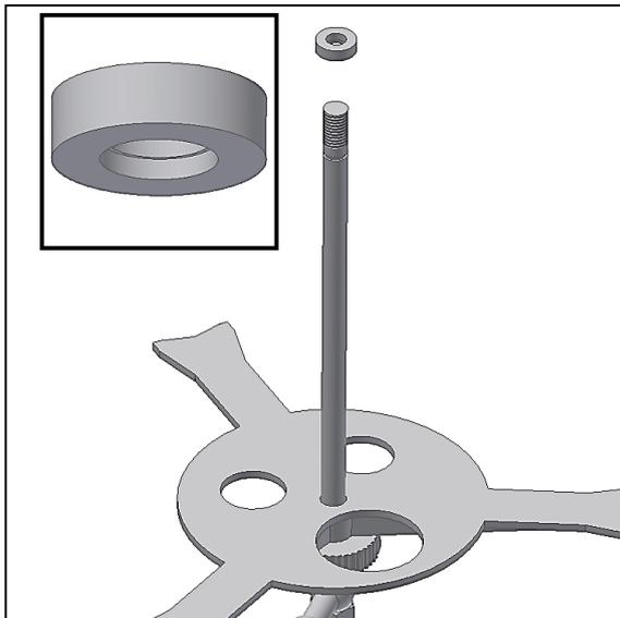
Figure 5. Slide supplied washer in the right direction.
