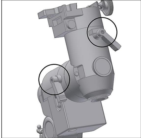
Figure 10. Clutch lockers.
