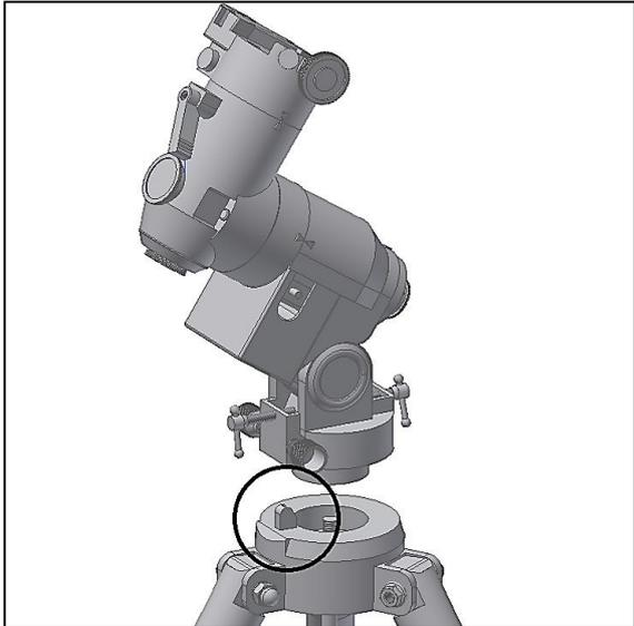
Figure 13. Align mount and tripod post.
