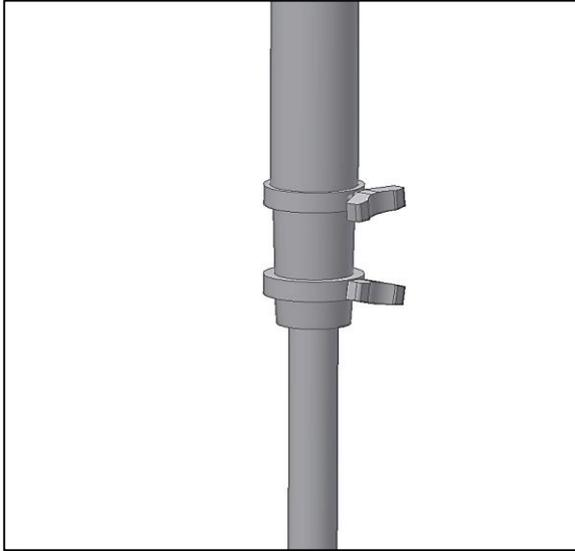
Figure 1. Extend the tripod's legs.
