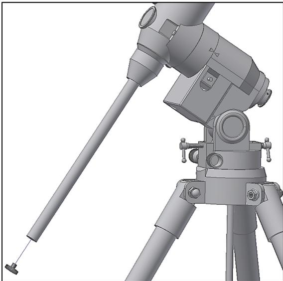
Figure 15. Remove foot saver to slide Counter-weight.
