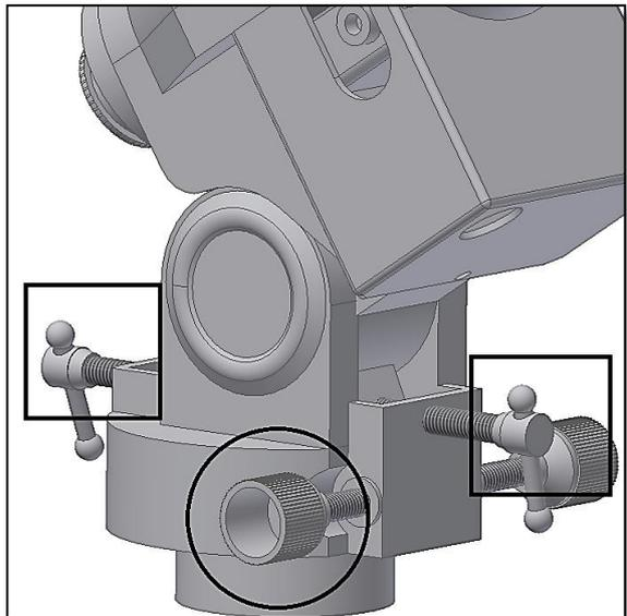
Figure 12. Altitude and azimuth hand-knobs.
