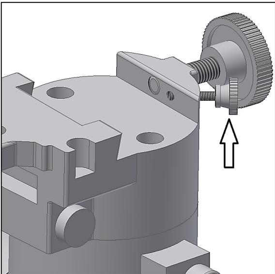
Figure 18. Use the safety locking thumbscrew.
