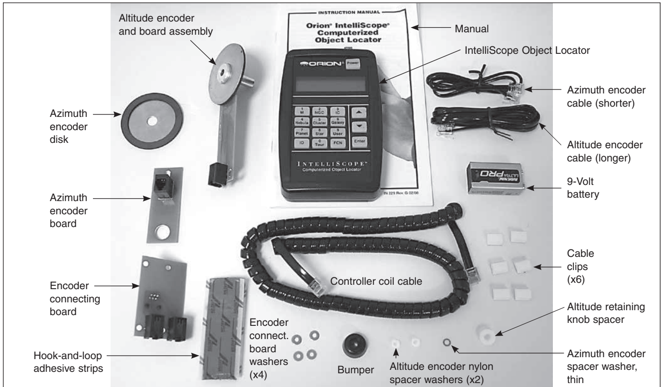
Figure 3. The parts contained in the IntelliScope Object Locator box.
