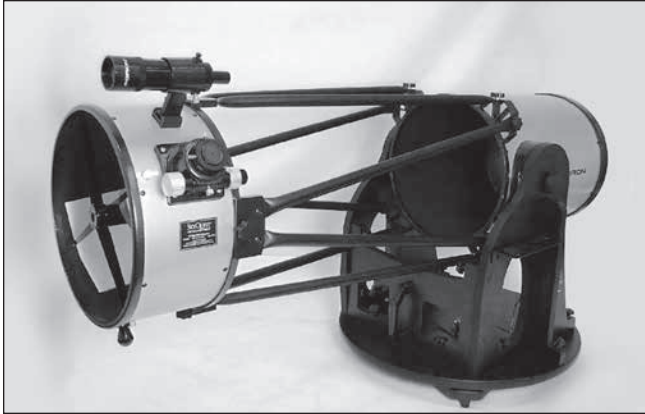
Figure 37. This image shows the XX14i properly set up for collimation. Note the white paper placed across from the focuser and the horizontal orientation of the optical tube. Ideally, the telescope should be pointing at a light-colored wall.
