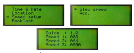
Press and hold ENT.  $\square$  Select "Speed setup" with Arrow keys  $\square$  ENT.  $\square$  Select "Slw speed" with Arrow keys  $\square$  ENT.  $\square$  Press and hold ENT.  $\square$  Change the speed of "Guide" with Arrow keys and keypad  $\square$  ENT. (completed)
