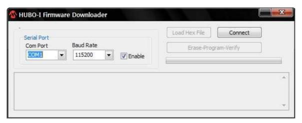
③ Execute the downloaded HUBO\_Firmware\_Loader.exe, select COM Port and click Connect. Baud Rate is 115200. Refer to 9. Conneting a PC to check the COM port.
