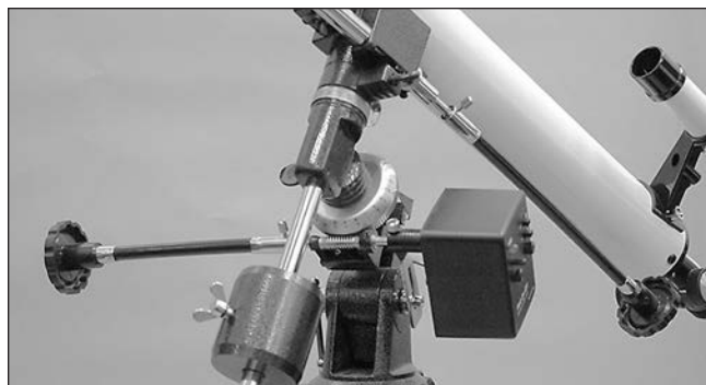
Figure 5: The AstroTrack installed on the EQ-1 mount.
