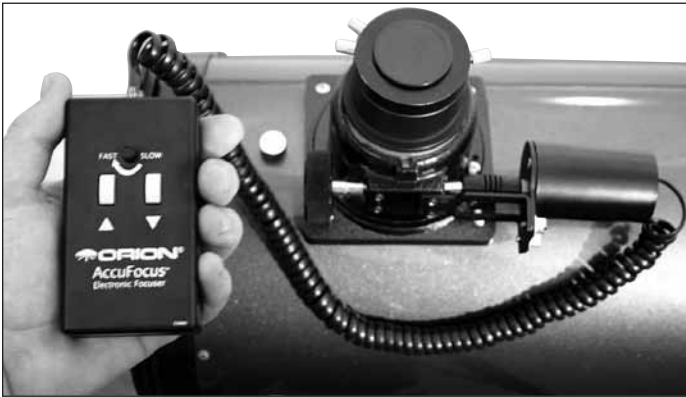
Figure 11. The assembled and installed AccuFocus Electronic Focuser.
