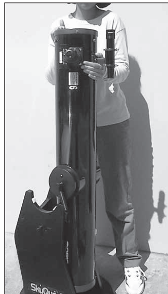
Figure 3. Set the optical tube on the "cradle" of the base so that the altitude side bearings on the tube rest on the white plastic "pads," and the finder is facing away from the front brace (Part B).
