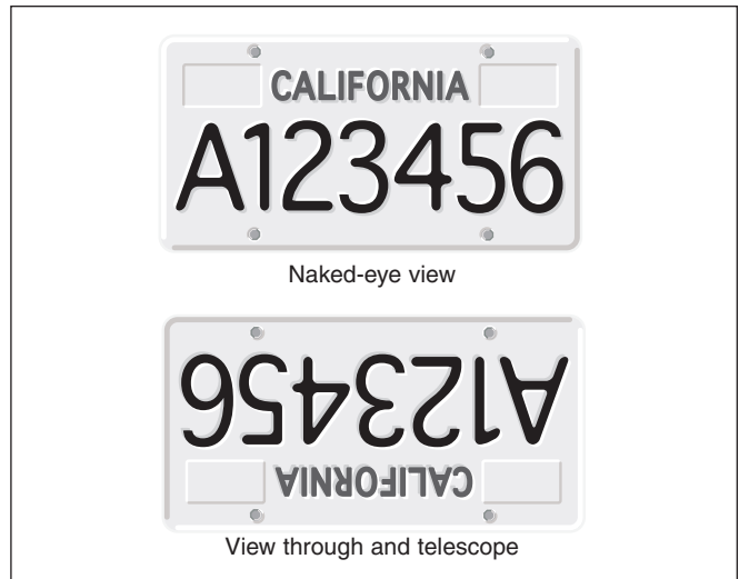
Figure 10. The view through a reflector telescope is upside down.
