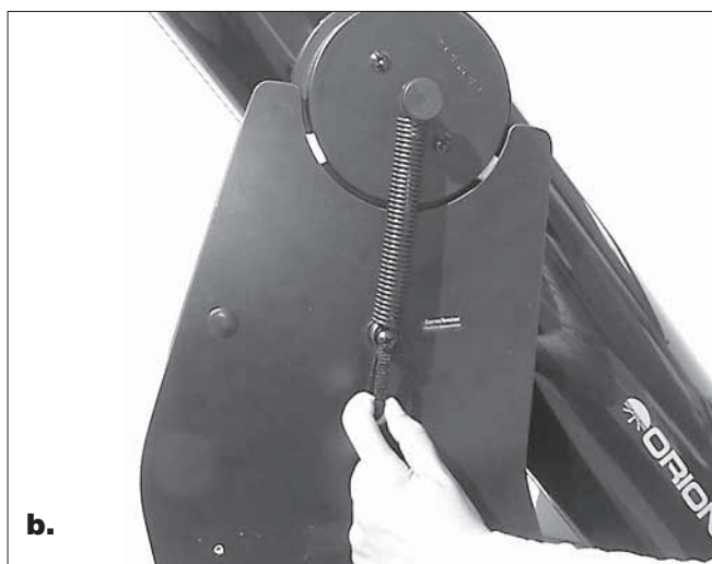
Figure 7. (a) To attach the spring to the base, grip the pull loop with your index finger and pull down on the spring. (b) While pulling down, slip the end ring of the spring over the bolt head and onto the narrow part of the nylon spacer, then release the pull loop.
