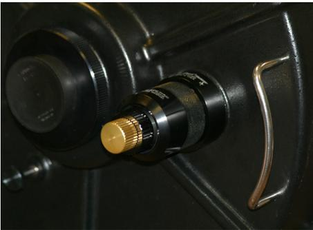
Thread the Knurled Sleeve onto the focuser in the opposite direction that it was removed. When transporting the telescope, reverse the sleeve to its original position to protect the focus knobs.
