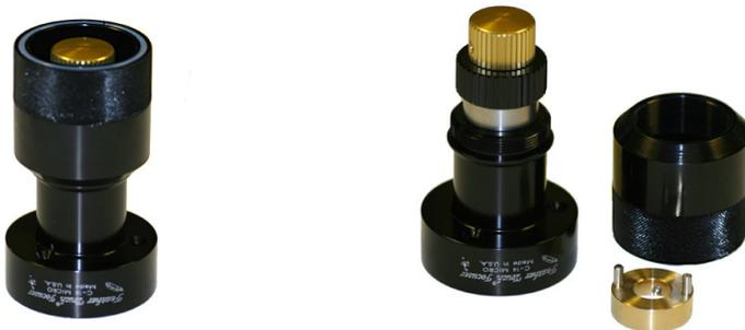
Begin by separating the 3 components of the SCT MicroFocuser. Remove the packing foam from the inside of the focuser. This will allow the Adapter Ring to drop out of the inside of the focuser. Remove the Knurled Sleeve from the main focuser. The Sleeve protects the focus knob during shipping and covers the mounting screws when the focuser is attached to the telescope.
