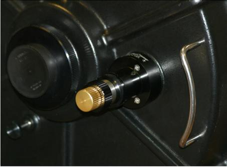
Slide the MicroFocuser over the Adapter Ring so the pins on the ring fit into the matching holes in the focuser. It may help to rotate the black focus knob slightly to get the pins into the holes. The three mounting holes in the base of the focuser should line up with those on the telescope. Secure the focuser using the included 3 Phillips-head screws.
