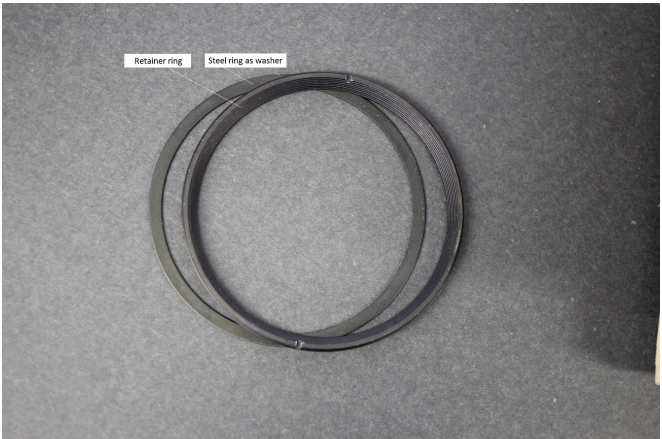
Fig. 7: Retainer ring with steel ring after removing
