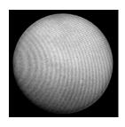
Another effect present in CCD imaging of monochrome light of Hydrogen Alpha is the interference pattern - or Newton's Rings. The effect is similar to interference testing of an optical surface between two flat surfaces. The sensor and cover slip cause a small interferometer inside the camera and cause a Newton's Ring moire' pattern. The CCD chip must be tilted to a minor degree to prevent this pattern. Recent advances
