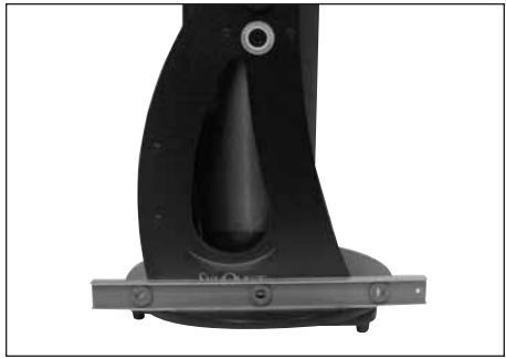
Figure 8. Place a carpenter's level on the base as shown. The base should stay level through a 180° rotation in azimuth. Once the vertical stop is set, the base does not need to be level to function properly.
